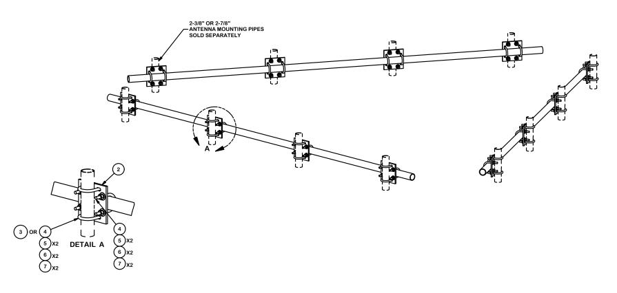
**TOLERANCE NOTES** TOLERANCES ON DIMENSIONS, UNLESS OTHERWISE NOTED ARE: SAWED, SHEARED AND GAS CUT EDGES (\$ 0.030") - NO CONING OF HOLES LASER CUT EDGES AND HOLES (\$ 0.030") - NO CONING OF HOLES BENDS ARE ± 1/2 DEGREE ALL OTHER MACHINING (± 0.030") ALL OTHER ASSEMBLY (± 0.060")
